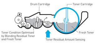
The lifetime of the drum cartridge depends on the effects of stress applied to the tone toner stress. Panasonic's new drum cartridge controls the amount of toner supplied to the drum cartridge by sensing the toner residual amount and optimises the proportion of fresh & residual toner in the drum cartridge
