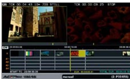
Playlist preparation example 1: Displaying player side and recorder side playback screens (with the player side selected)
